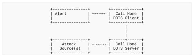
Figure 2: Basic DOTS Signal Channel Call Home Functional Architecture
