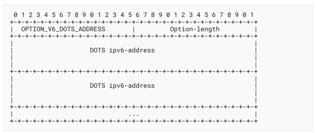
Figure 5: DHCPv6 DOTS Address Option
