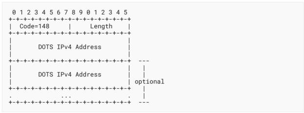
Figure 7: DHCPv4 DOTS Address Option
