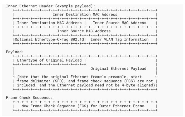
Figure 3: Geneve Packet Format over IPv6
