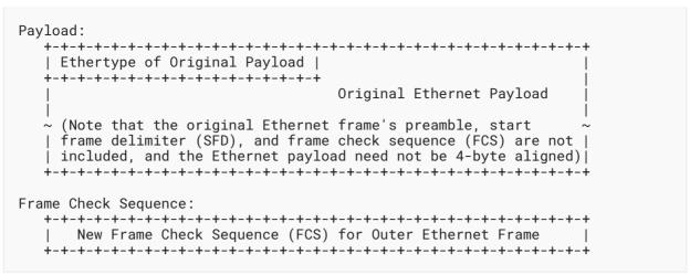
Figure 2: Geneve Packet Format over IPv4
